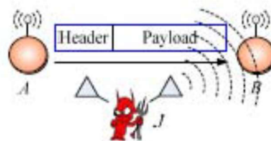
Figure (a): Realization of a selective jamming attack
