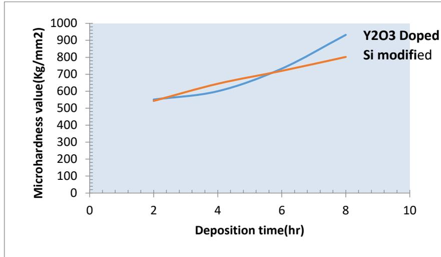
Fig.(8) Vickers micro-hardness vs. deposition times.
