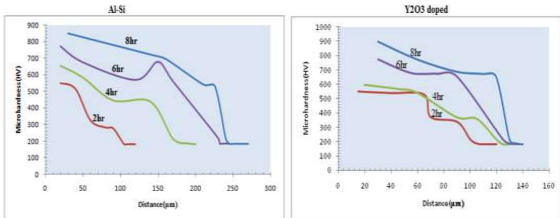
Fig. (9) Vickers micro-hardness vs. depth for different coating times(Al-Si and Al-Si-Y<sub>2</sub>O<sub>3</sub>).
