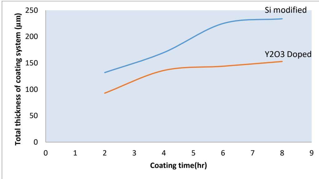
Fig. (6) Average total thickness of the two types of coating.
