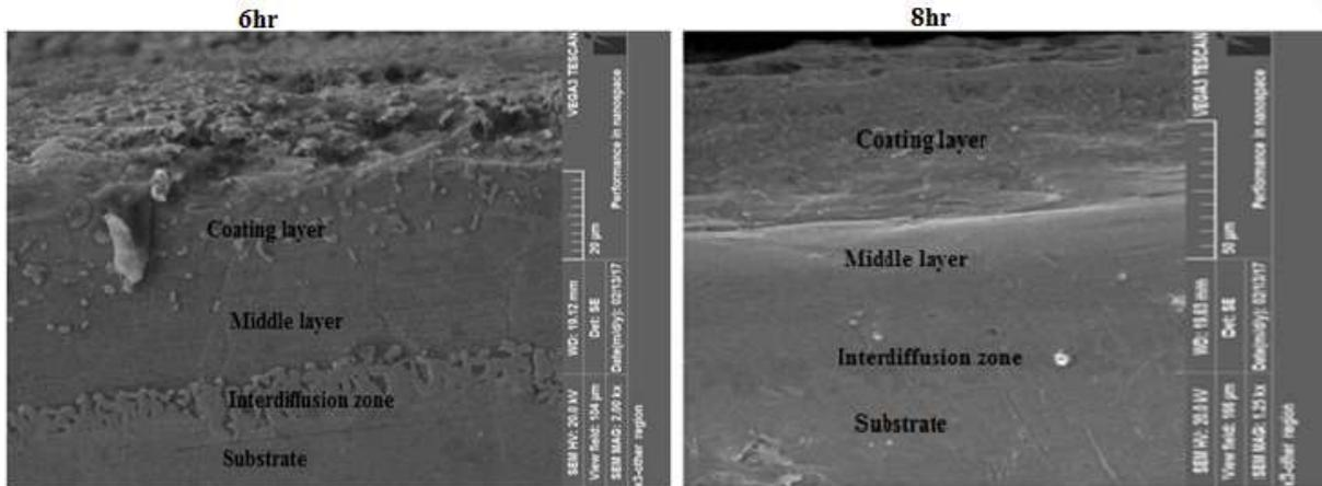
Figure (3) Microstructure of ytria doped silicon modified aluminide diffusion coating of Inconel 600 at 1120°C for (a- 2hr, b-4hr, c-6hr, d-8hr).
