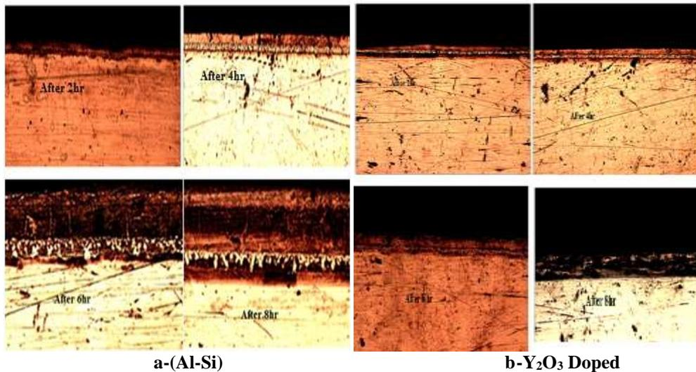
Fig.(7) LOM show the increases thickness of coatings layer with deposition time.
