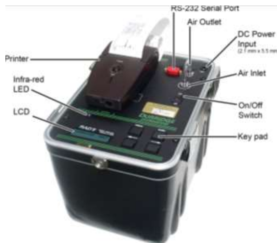
Figure 3. Radon measuring apparatus : RAD7
