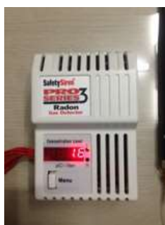
Figure 2. Safety Siren PRO 3 radon detector
