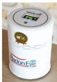
Figure 1. Ion chamber-type radon counter : RD200 (model: SN242)
