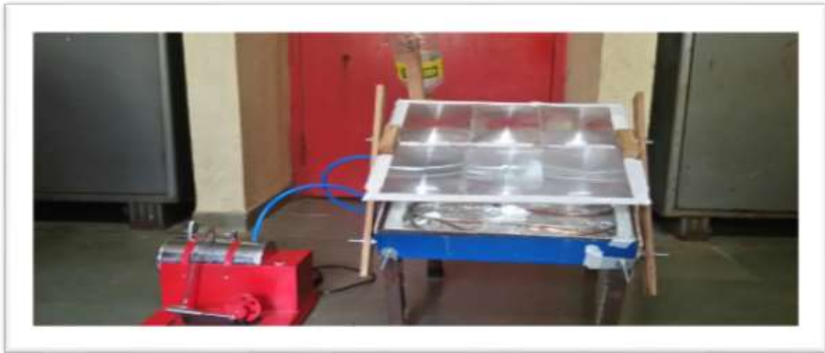
Fig 5: Solar engine with Fresnel lens
