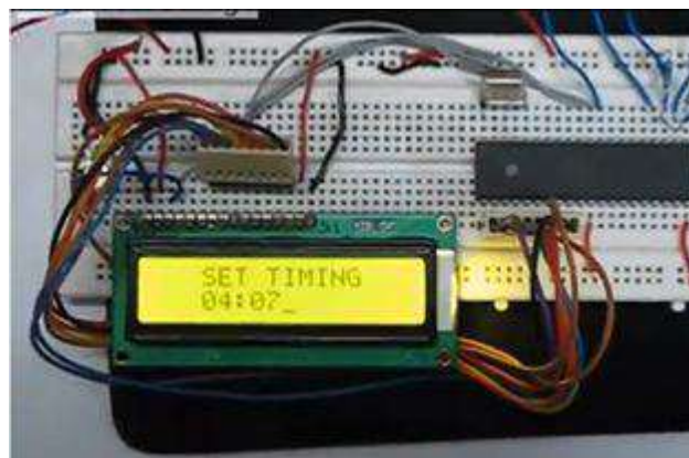
Fig 6. Implementation of Digital Clock on Breadboard.
