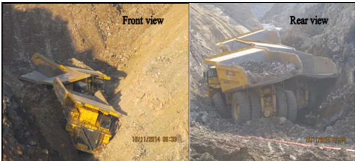
Figure 2: Three 240t Komatsu 830E trucks partially buried after the slough at Nchanga Open Pit
