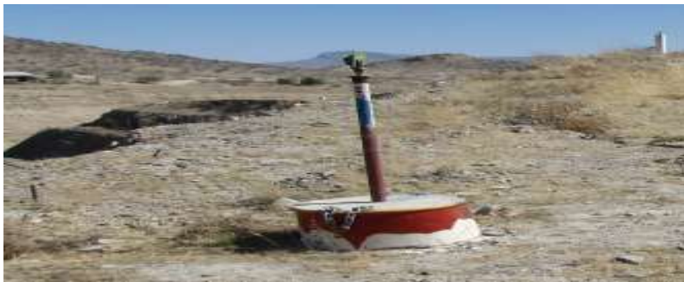
Figure15: Illustration of target and prism used at NOP foot wall slope
