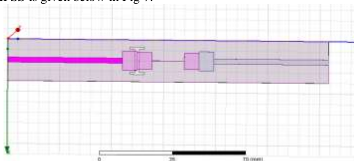
Fig 7. Tri-section stepped impedance filter structure with I- shaped DGS modelled using HFSS
