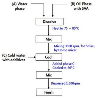
Figure 4. Preparing method of fine emulsion with botanical oil complex using PIT self assembly system without high pressure homogenizer.
