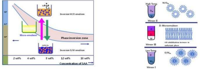
Figure 1. Mechanism of phase inversion zone depend on the temperature with (POE)12~20 fatty acid ethers of nonionic surfactants. Figure 2. Phase prism, Winsor systems, and dispersion structure of an emulsion composed of nonionic surfactant, oil, and water depend on the various temperatures.
