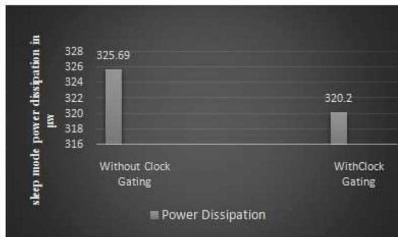
Fig. 8(b). Sleep mode Power dissipation with and without Clock Gating.
