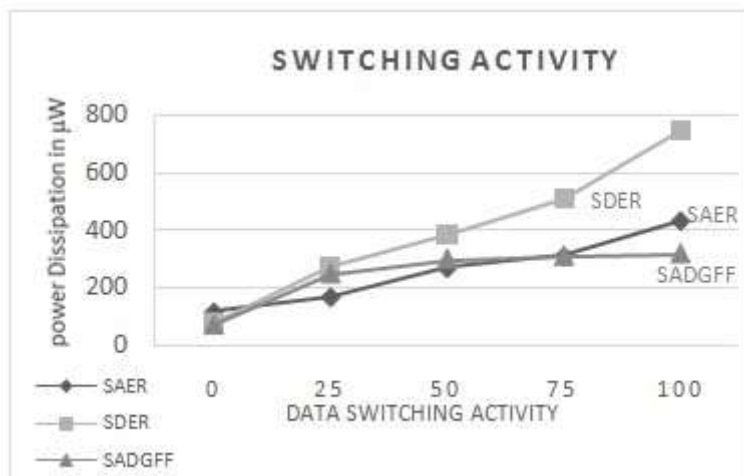
Fig. 7(b). Power dissipation PD at various Switching activity.
